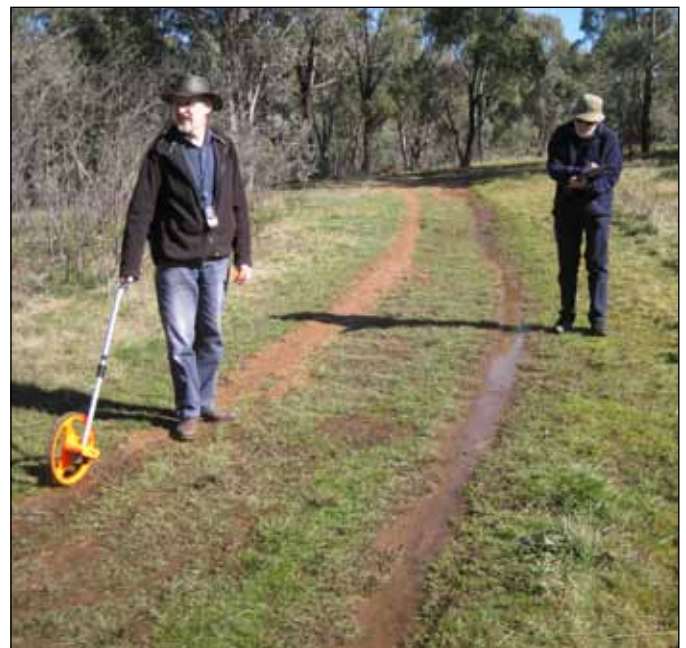
Warren Bond and Geoff McAlpine conducting track erosion assessments
